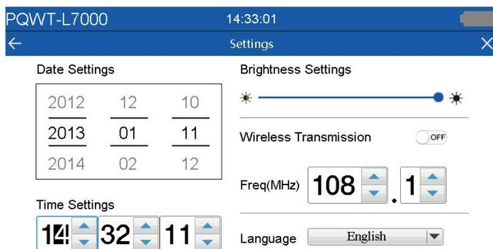
Wireless transmission: It can be received by USING FM radio or mobile phone headphones with FM radio function. It is convenient for multiple people to listen at the
